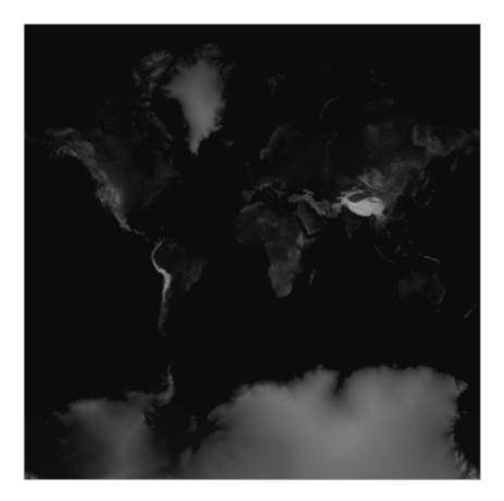
A <u>raster layer</u> is made of a grid where each cell is called a pixel and has a numeric value. In the case of the **Terrain** layer, the value of each pixel represents elevation in meters. The pixels with the highest values, such as the highest mountain peaks, appear in white. The pixels with the lowest values, such as land depressions below sea level, appear in dark gray or black.
