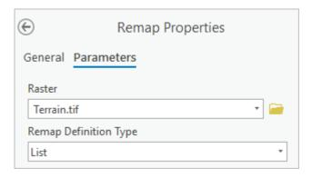
In the **Remap** table, you'll define the reclassification rules. Based on the legend for the **Terrain.tif** layer in the **Contents** pane, you can see that the lowest value possible for that layer is about **-22.9** meters and the highest is **96.5** meters.
