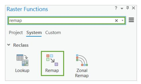
The **Remap Properties** pane appears. The **Remap** tool allows you to change or reclassify the pixel values of a raster and produce a new raster layer with the new values.
