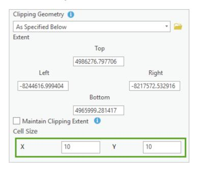
The cell size determines the resolution of the output raster. In this case, each pixel will cover a piece of the earth that is 10 meters by 10 meters, or 100 square meters.
